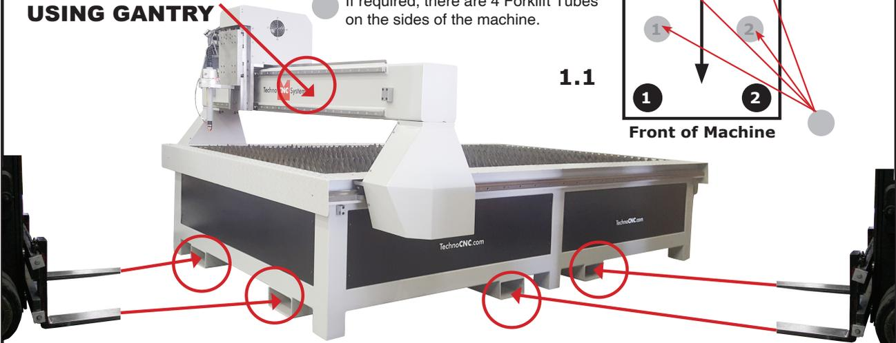
**NOTE: Forklift capacity must be adequate to safely lift the machine.**
